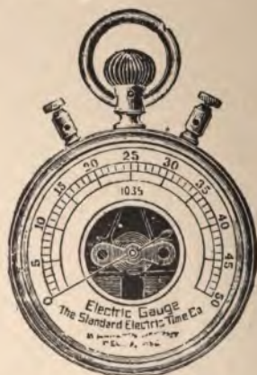
FIG. 223.—Pocket battery gauge. Such an instrument is indispensable to every electrician but the readings of its records must first be determined by some known standard, since they are purely arbitrary.
